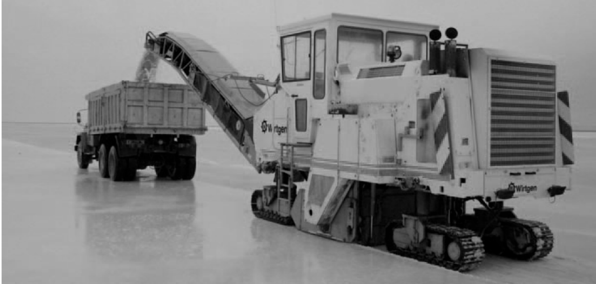
Figure 3. Modified cold milling machine 2000 DC developed in Turkey for salt production.
