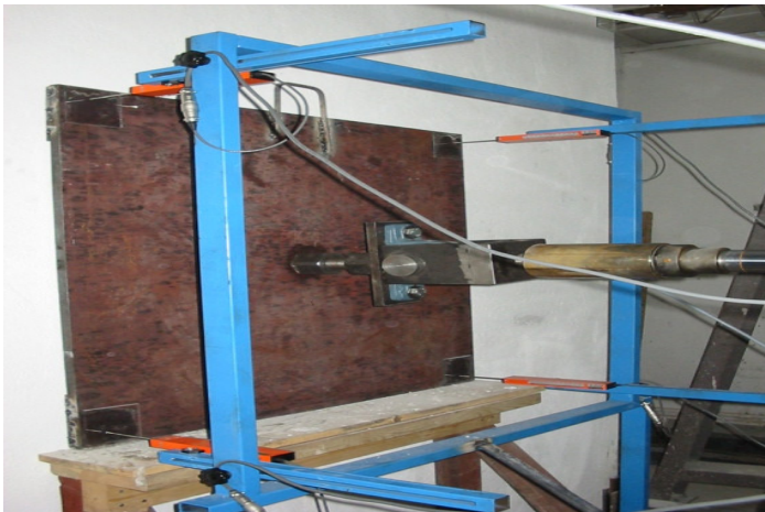
Figure 12. The location of loading plate and LVDTs.
